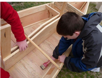
Cutline on attached photo: Students use scrapers to finish deck of a “Watermen's 15” -- a 19 th century sailing skiff.
